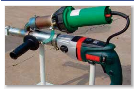
▶ Extrusion Plastic Welding
